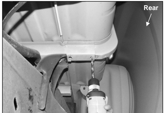
(Fig 11) Use 1/2" drill bit to open blocked off hole in bed support. Do not drill through bottom of bed
